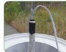
The light sensor is attached to the screw.
