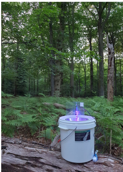
Figure 5. LED trap using power bank and sensor designed by Vlinderstichting.
