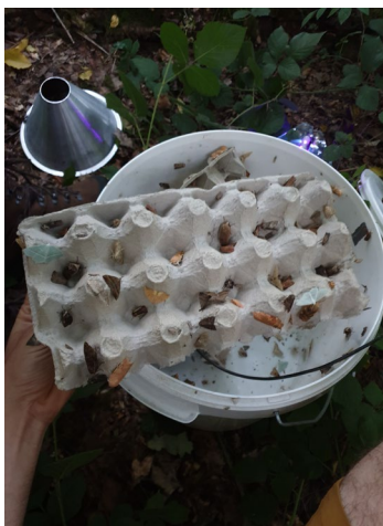
Figure 5. LED trap using power bank and sensor designed by Vlinderstichting.
