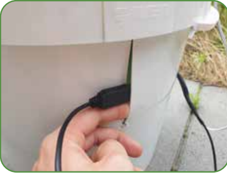
Open the slot slightly with your fingers to allow the USB connector to pass through.
