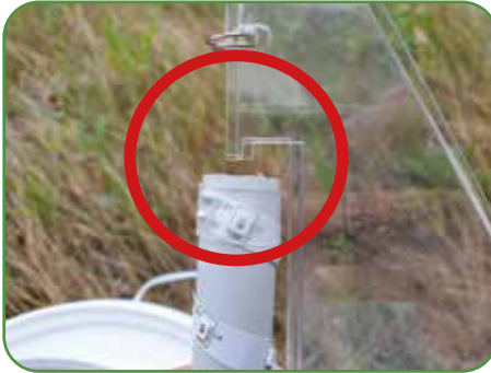
Slide the tube over the tips of the plates.
