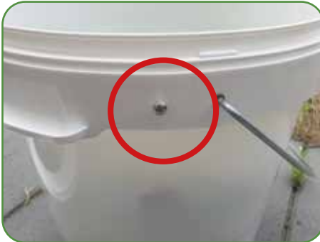
This is the screw for the light sensor.
